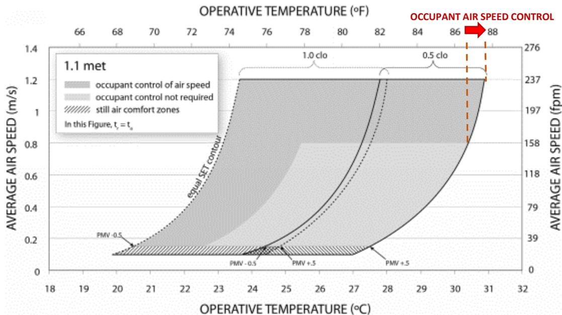
ASHRAE Standard 55 Figure 5.3.3A – Acceptable ranges of operative temperature and average air speed for comfort zone presented in Figure 5.3.1 at humidity ratio 0.010.
